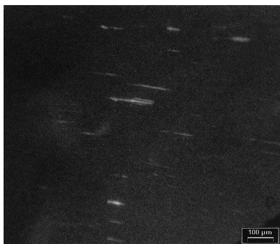
Figure 2. Microtome pellet cut showing „white spots“ in a coloured PE pipe grade.
